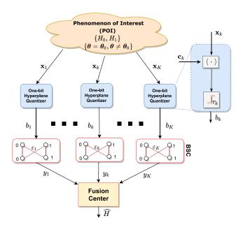
Fig. 1. System model used in this paper. Each sensor compresses its measurement vector via a hyperplane-based quantizer. Each bit is then sent through a binary symmetric channel and received by the FC.
