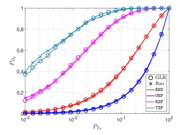
Fig. 2.  $P_{D_0}$  vs.  $P_{F_0}$  for GLR (o markers) and Rao (× markers) tests. Random (RND), uniform (UNF), random subspace (RSP) and top subspace (TSP) precoding approaches are compared. WSN with K=15 sensors, m=8 and p=3, and the sensing SNR = 5 dB. One bit-quantization ( $m_k=1$ ) and ideal BSCs are considered ( $P_{e,k}=0$ ).
