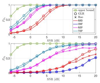
Fig. 3.  $P_{D_0}$  vs. SNR [dB] for GLR (o markers) and Rao (× markers) tests, subject to  $P_{F_0}=0.01$ . Top and bottom plots refer to two-bit  $(m_k=2)$  and one-bit quantization  $(m_k=1)$ , respectively. Random (RND), Uniform (UNF), Random Subspace (RSP) and Top Subspace (TSP) precoding approaches are compared. WSN with K=15 sensors, m=8 and p=3. Ideal BSCs are considered  $(P_{e,k}=0)$ .
