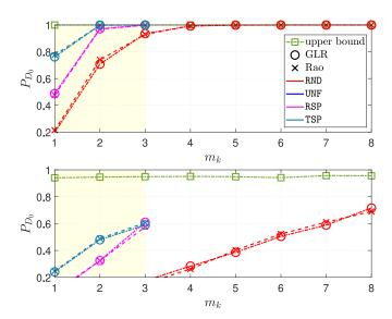
Fig. 4.  $P_{D_0}$  vs.  $m_k$  for GLR (o markers) and Rao (× markers) tests, subject to  $P_{F_0}=0.01$ . Top and bottom plots refer to SNR = 5 dB (moderate SNR) and SNR = -3 dB (low SNR), respectively. Random (RND), uniform (UNF), random subspace (RSP) and top subspace (TSP) precoding approaches are compared. Shaded area indicates number of quantization bits  $\leq$  of the signal subspace size. WSN with K=15 sensors, m=8 and p=3. Ideal BSCs are considered ( $P_{e,k}=0$ ).
